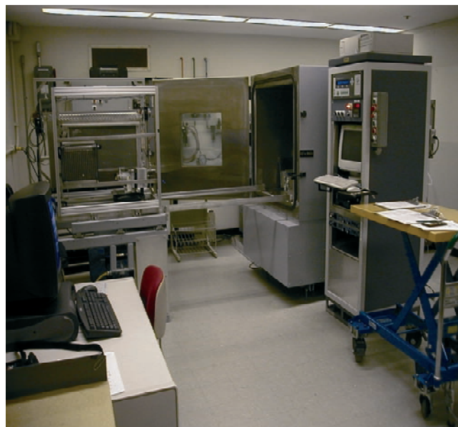
Figure 1. Test setup at Delphi Thermal & Interior Technical Center, Lockport, NY. The 1314 instrument is mounted in the top of the rack system to the right
